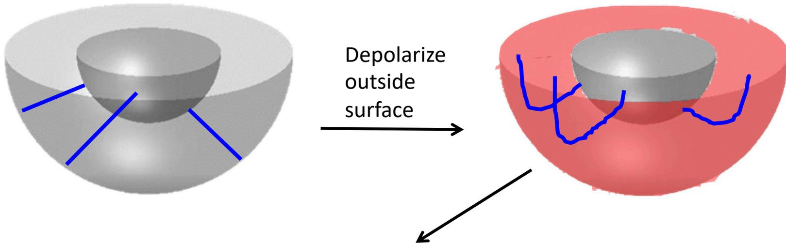
All filaments are converted into C-shaped or U-shaped filaments! These should all shrink and disappear.
