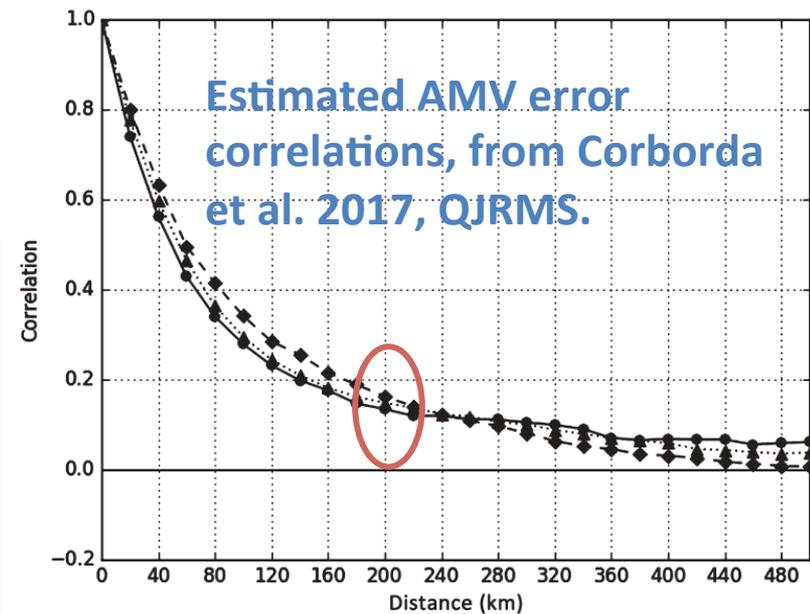
Figure 5. AMV wind-speed observation horizontal error correlation function estimate (20 km bin size) for the three SEVIRI channels, IR108 (solid with circles), WV062 (dashed with diamonds) and WV073 (dotted with triangles), at high level.
