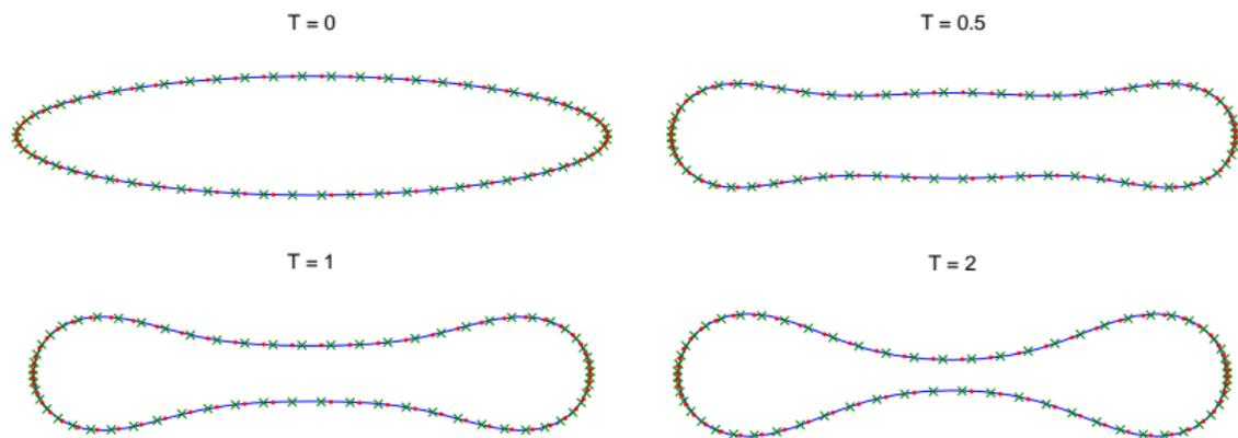
**Figure:** Freely suspended vesicles with different penalty number  $\sigma_0$ . Blue solid line:  $\sigma_0 = 2 \times 10^3$ ; green marker “x”:  $\sigma_0 = 2 \times 10^4$ ; red marker “.”:  $\sigma_0 = 2 \times 10^5$ .
