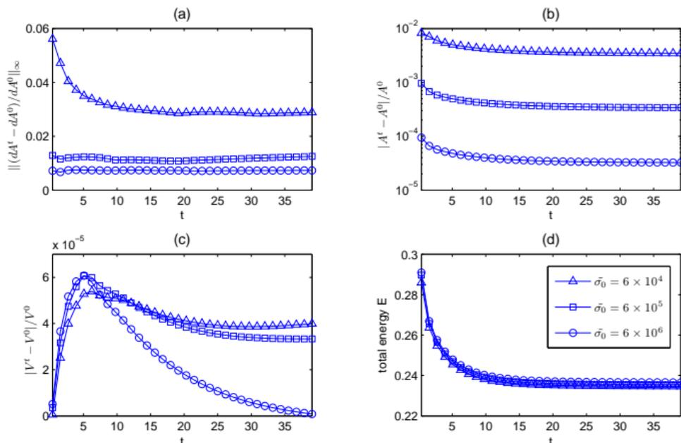
Figure: The comparison for three different stiffness parameters:  $\sigma_0 = 6 \times 10^4$  ( $\Delta$ ),  $6 \times 10^5$  ( $\square$ ), and  $6 \times 10^6$  ( $\circ$ ). (a) the maximum relative error of the local surface area; (b) the relative error of the global surface area; (c) the relative error of the global volume; (d) the total energy.
