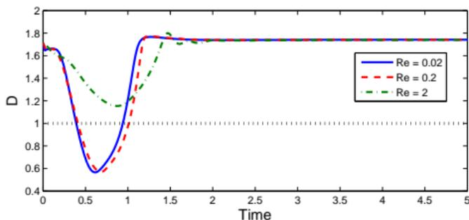
**Figure:** The time evolutionary profile of deformation number  $D$  for  $Re = 0.02, 0.2, 2$  with fixed  $C = 0.1$  and  $G = 0$
