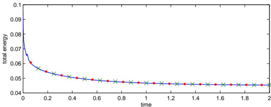
Figure: The corresponding evolution of total energy. Blue solid line:  $\sigma_0 = 2 \times 10^3$ ; green marker “x”:  $\sigma_0 = 2 \times 10^4$ ; red marker “.”:  $\sigma_0 = 2 \times 10^5$
