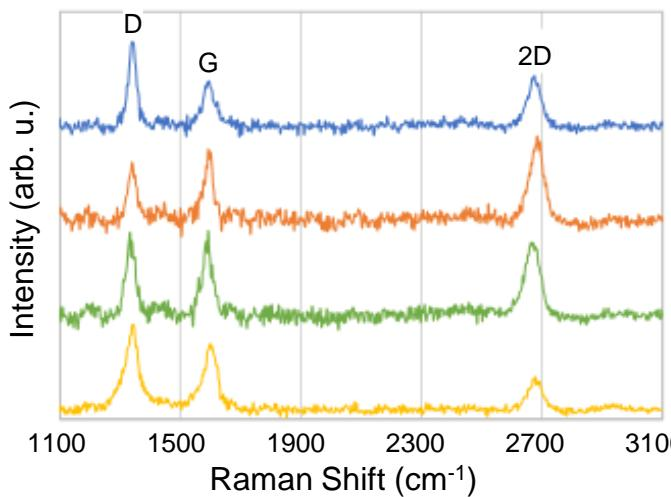
Graphene cap formation on 300 mm wafers
