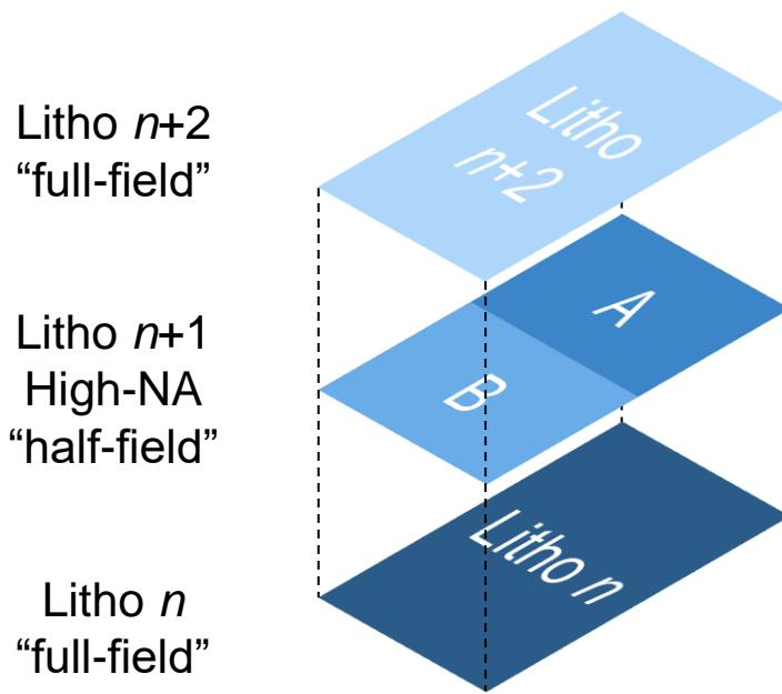
Low-NA and High-NA mix-and-match printing will introduce new overlay error components
