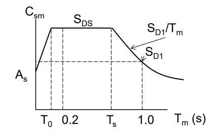
Problem 61: Using the uniform load method for the transverse response, determine the equivalent seismic load.  $C_{sm}$  = 1.21, W = 1,200 k, and L = 120 ft.
