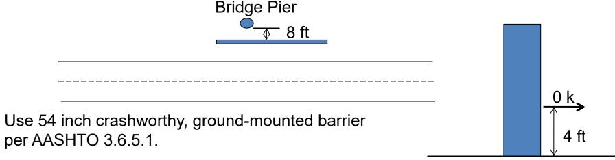
Note that a 42 inch high barrier is permitted when the separation distance exceeds 10 feet
