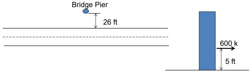
Note that 600 k load is horizontal and application must consider all angles between 0 to 15 degrees with the edge of pavement.
