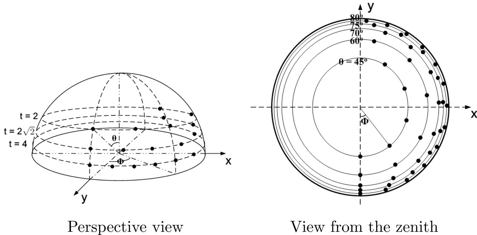
Figure 8: It is enough to simulate five tilts  $\sqrt{2}, 2, 2\sqrt{2}, 4, 4\sqrt{2}$  and a growing but moderate number of longitudes per tilt. **The overall simulated image area is five times the original.**
