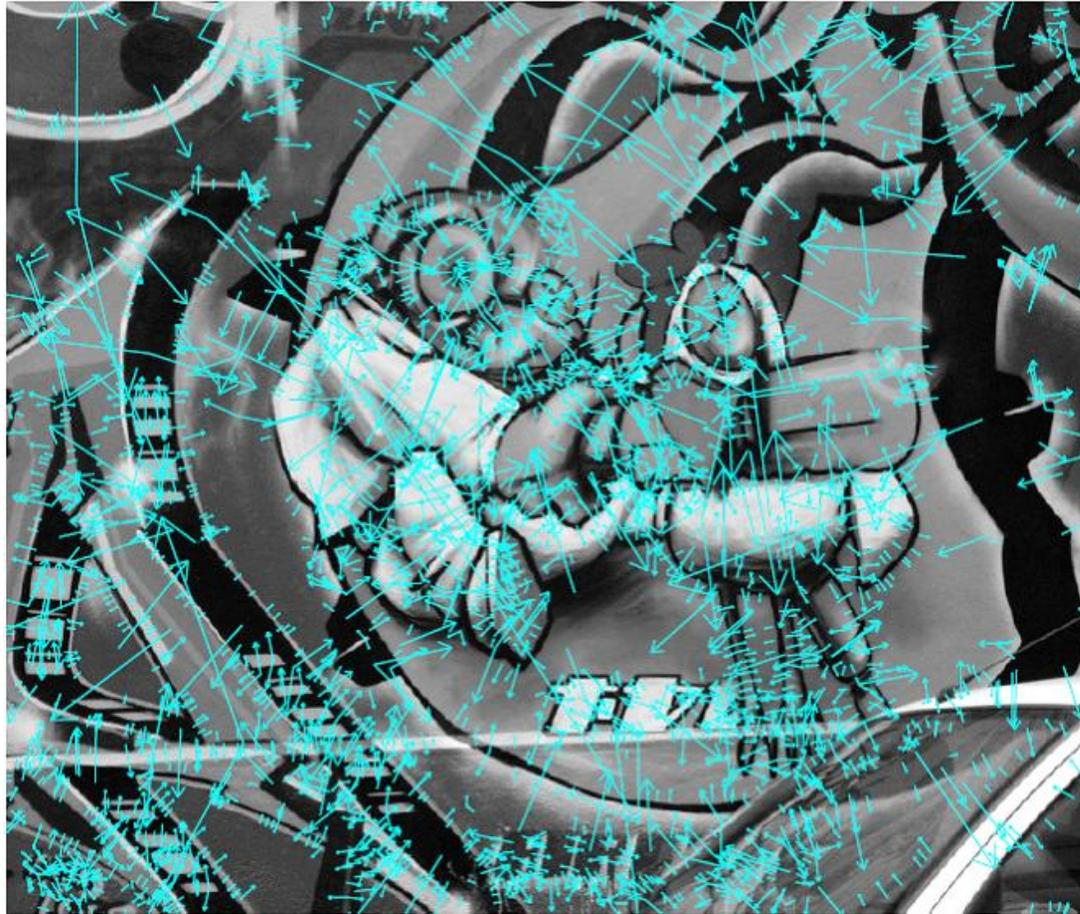
Figure 6: SIFT key points (scale and orientation). Each one is covariant or invariant with respect to: translation, rotation, scale, and contrast changes (6 parameters out of 8)
