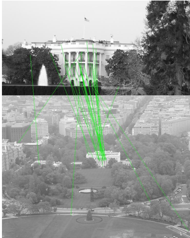
Figure 1: Recognition with extreme scale difference. 26 matches, 6 outliers. Exp. : Rabin, Gousseau, Delon, SIFT method
