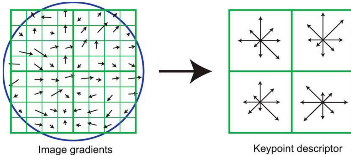
Figure 5: Each key-point is associated a *square image patch whose size is proportional to the scale and whose side direction is given by the assigned direction*. Example of a  $2 \times 2$  descriptor array of orientation histograms (right) computed from an  $8 \times 8$  set of samples (left). The orientation histograms are quantized into 8 directions and the length of each arrow corresponds to the magnitude of the histogram entry.
