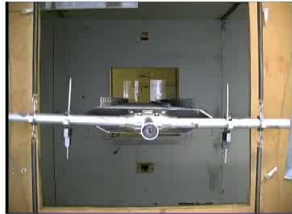
Vortex-induced vibrations in a section model of Hardanger Bridge, Norway
