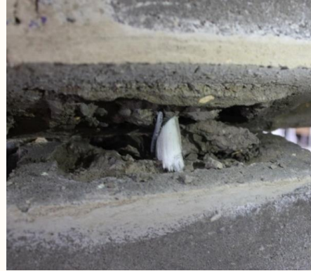
GFRP Rupture Tension-Controlled Section
