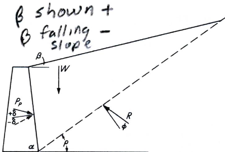
Note: Beta (the slope angle is shown positive, it can also be negative (i.e. a falling slope), the angle  $\rho$  is equal to  $45 - \phi/2$
