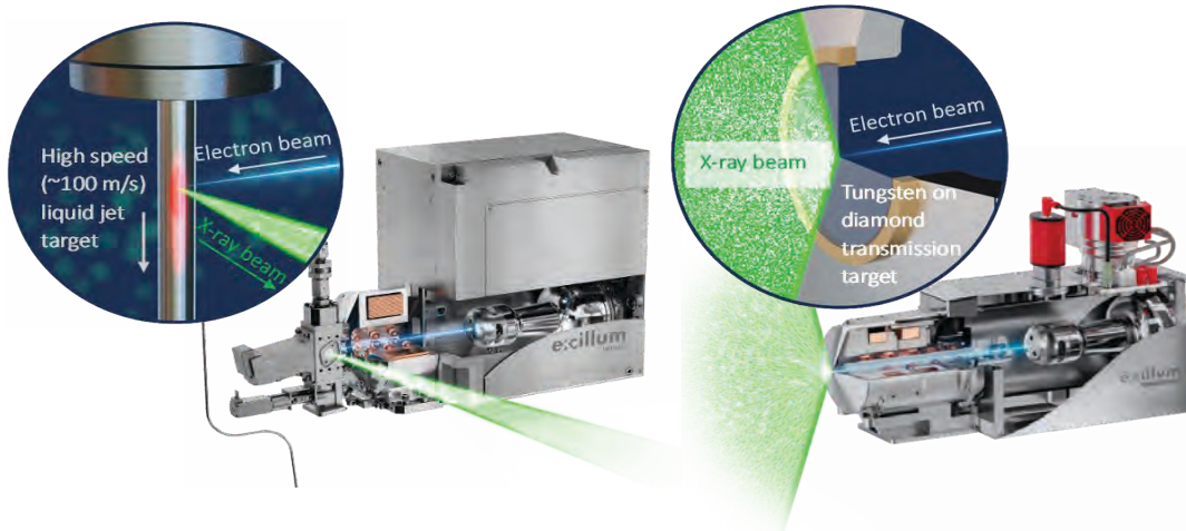
FIGURE 1. Illustration of MetalJet (left) and NanoTube (right) X-ray source technology.
