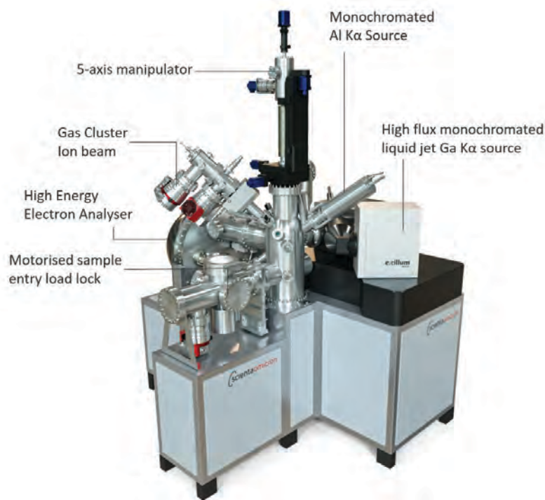
FIGURE 2. DeepCore-X redefines laboratory-based HAXPES by combining deep probing capability, automated high-throughput workflows, and operando measurement support. Its modular design and robust performance make it an indispensable tool for semiconductor interface research, bridging the gap between surface analysis and full device stack characterization – without the need for synchrotron access.
