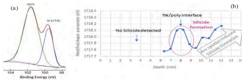
FIGURE 4. (a) XPS Si2p spectrum indicating the presence of SiON and Si-Si or silicide and (b) modified Auger parameter of Si vs. depth determined by HAXPES aided with Ar + sputtering reveals the presence of ~1nm silicide layer at the TiN/Si interface.
