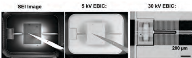
FIGURE 2. EBIC measurements, top-down, on IGBT device. At higher beam landing energy, imaging of sub-surface depletion zones is possible.
