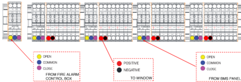
TERMINAL BLOCK WIRING DETAIL
