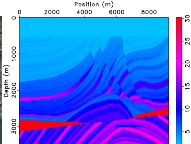
Left: Outcrop, Stuart I., WA (WS, 8/11). Right: Marmousi synthetic model (IFP 89): bulk modulus map  $\kappa$ , unit = GPa (density = 1 g/cm<sup>3</sup>)
