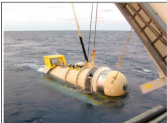
Figure 1: BP's Wolfspär<sup>®</sup> prototype low-frequency seismic source being retrieved during operational testing at the Gulf of Mexico systems integration test in 2014.
