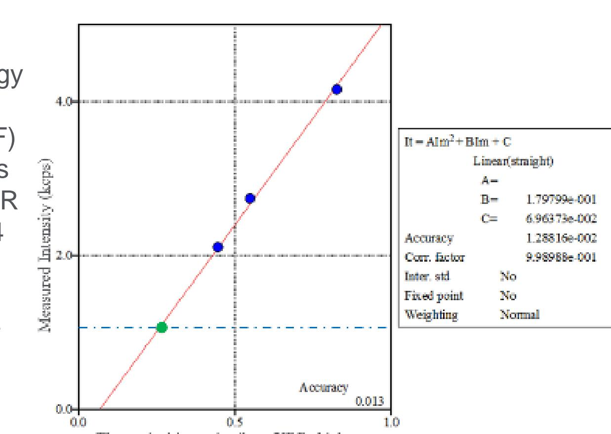
Fundamental parameter method calibration between calculated intensities and WDXRF measured counts.
