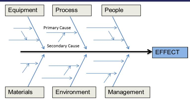
The various causes are grouped into categories (such as equipment, materials or processes) and the arrows in the image indicate how the causes cascade or flow toward the non-conformity.
