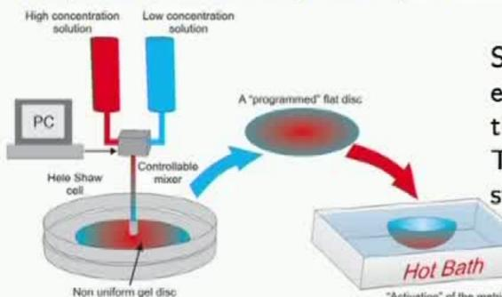
Shrinking by a different ratio  $\eta(r)$  at each radius r both in the radial and the azimuthal directions.
