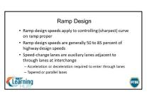
usually in the mid- to upper-range; however, the minimum design speed for direct connections is generally 40 mph (60 km/h).
