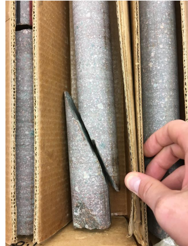
Near-vertical fracture in basement section of SHADS core
