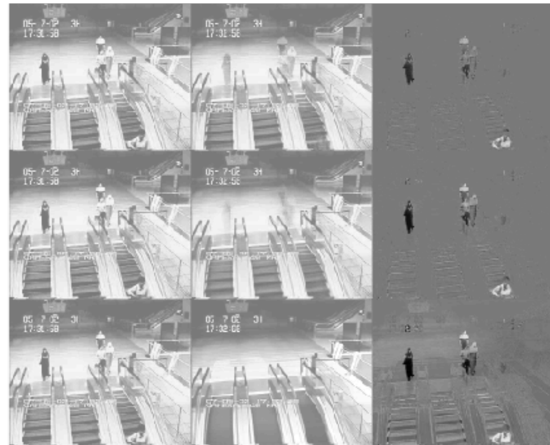
(b) X,L, and S matrices found by (from top to bottom) FPCP, IALM, and LMaFit.
