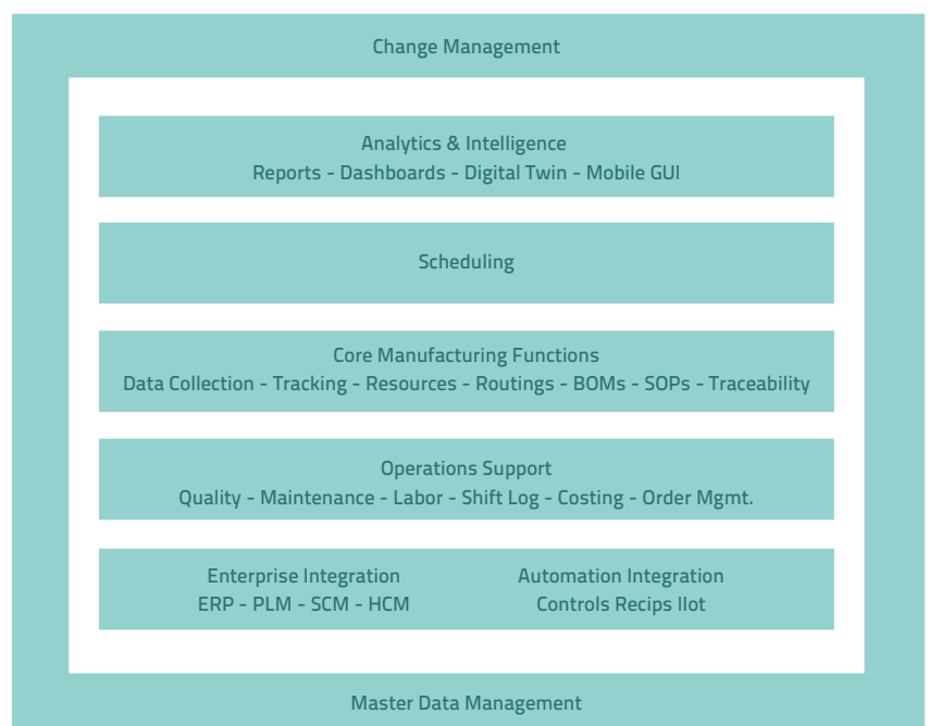
Figure 2 MES does provide connection to devices and to other applications, but in the middle, it's a rich set of functions to manage and optimize production operations.
