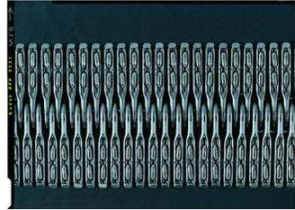
10. A solid plate butt joint compression belt splice. Like the bolt hinge, special bolts and nuts are used to compress the plates into the belt surfaces. These fasteners are generally used for the heavier bulk haulage applications where a sift-free, more permanent belt installation is needed. Only simple hand tools are needed for installation.
