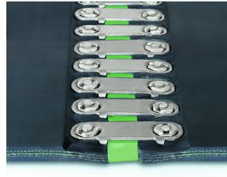
11. A solid plate butt joint compression belt splice for medium- to high-tension bulk haulage applications. Special rivets are driven through the belts without pre-punching holes. These fasteners are generally used for applications where a sift-free, more permanent belt installation is needed.
