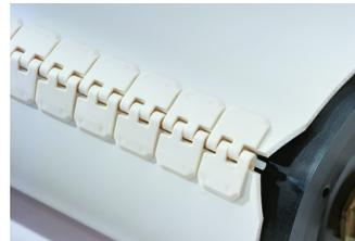
7. A heavy-duty bolt hinge fastener for bulk haulage applications. Commonly used in low- to medium-tension industrial belts requiring a hinged splice. The fastener plates are compressed into the belt by special bolts and nuts. Only simple hand tools are needed for installation.
