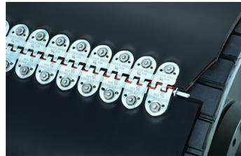
8. A heavy-duty riveted hinge fastener for medium- to high-tension bulk haulage applications. Available in several types of rivets and fasteners. Special rivets are driven through the belts, without pre-punching holes, to compress the fastener plates into the belt.
