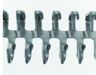
4. A light- to medium-duty hinged plate fastener that derives its strength by the compressive clamping action of either rivets or staples. Provides stronger splices in most types of belts.
