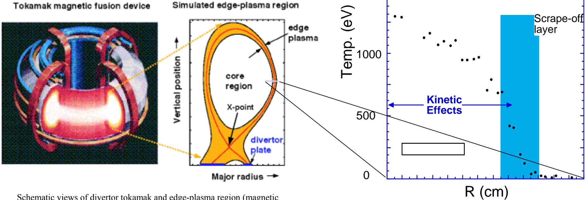
Schematic views of divertor tokamak and edge-plasma region (magnetic separatrix is the red line and the black boundaries indicate the shape of magnetic flux surfaces)
