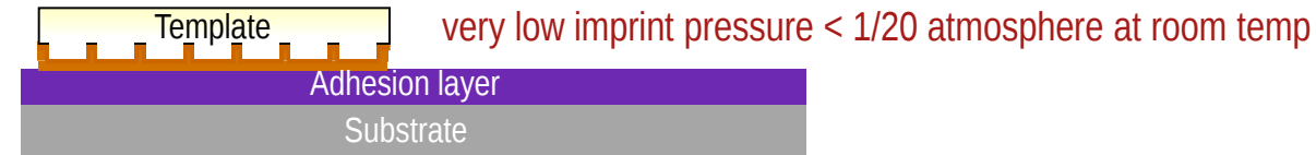
Step 2: Lower template and fill pattern
