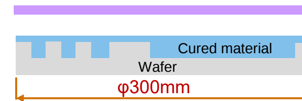
Step 3. UV Cure and Separation
