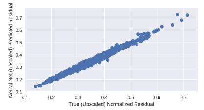
Figure: The fine grid residual norm vs neural net filter residual norm with continuous learning
