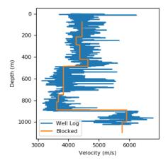
Figure: The well log (blue, courtesy of Pioneer Natural Resources) and 9-layer block (orange).
