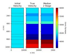
Figure: The initial, true, and median velocity fields for the neural net two stage MCMC. The dashed lines in the initial velocity picture mark the positions of the pre-set interfaces.
