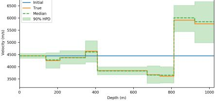
Figure: A one-dimensional slice of the velocity field in depth.
