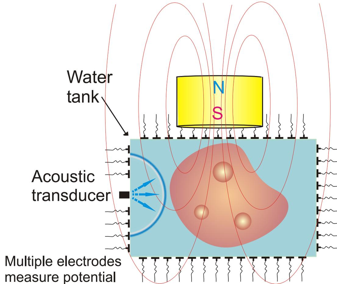
Ultrasound makes electrons and ions vibrate.
