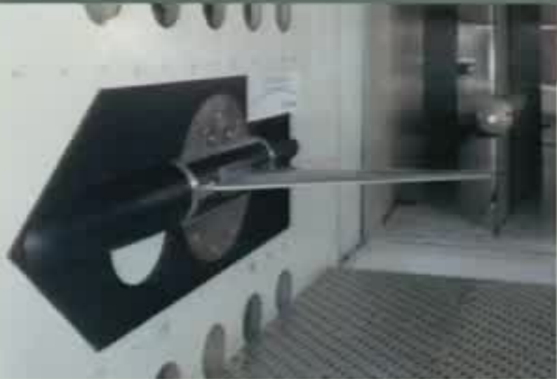
Transonic wing in ONERA S2MA wind tunnel
