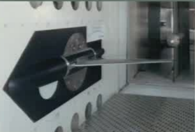
Transonic wing in ONERA S2MA wind tunnel
