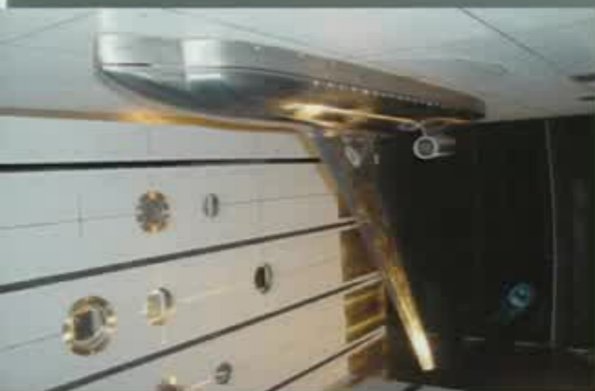
Cryotechnic test of generic Falcon shape in ETW
