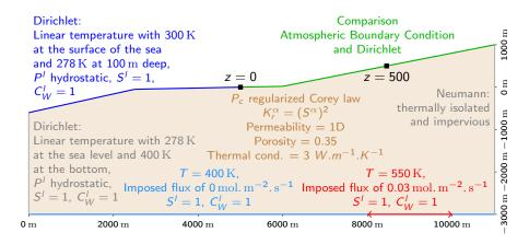
Liquid density and viscosity are fixed to prevent thermal instabilities.
