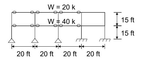
Problem 16: Determine the first mode shape for the system shown. All columns are W10×45. All beams and columns are oriented for strong axis bending in the plane of the figure. Also, assume that the moment frame beams are infinitely stiff (i.e.,  $I_x = \infty$ ) so that columns respond as fixed-fixed columns.
