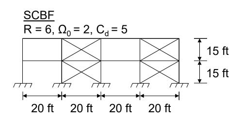
Problem 8: Using the equivalent lateral force method (Section 12.8 of ASCE 7-10), determine the base shear V for the special steel concentrically braced frame office building shown.  $S_{DS} = 1.0$ ,  $S_{D1} = 0.43$ ,  $S_{1} = 0.40$ . The structure is to be located in Charleston, SC.
