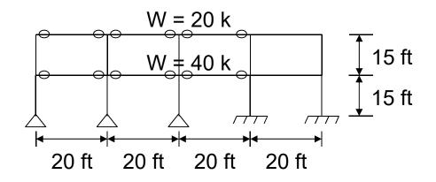
Problem 14: Determine the eigenvalue equation for the system shown. All columns are W10×45. All beams and columns are oriented for strong axis bending in the plane of the figure. Also, assume that the moment frame beams are infinitely stiff (i.e.,  $I_x = \infty$ ) so that columns respond as fixed-fixed columns.
