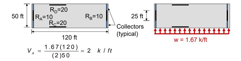
Problem 35: For the building plan view shown below and a total force V = 200 kips distributed across the building as shown, determine the maximum axial force (k) in the collector associated with wall A. Wall rigidities (stiffnesses) shown in the figure are in kips/ft. Assume a flexible diaphragm.
