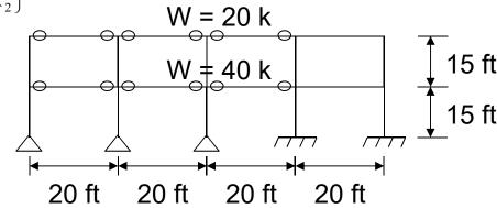
Problem 15: Determine the natural periods for the system shown. All columns are W10×45. All beams and columns are oriented for strong axis bending in the plane of the figure. Also, assume that the moment frame beams are infinitely stiff (i.e.,  $I_x = \infty$ ) so that columns respond as fixed-fixed columns.
