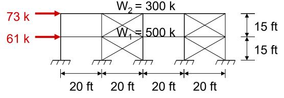
Problem 11: Using principles of dynamics, determine the natural period of the structure shown. All columns are W10×45. All beams and columns are oriented for strong axis bending in the plane of the figure. Also, assume that the moment frame beam is infinitely stiff (i.e.,  $I_x = \infty$ ) so that columns respond as fixed-fixed columns.
