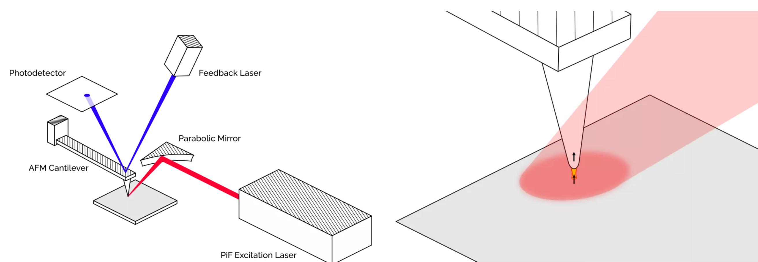
IR-AFM (or PiFM - Photo-induced Force Microscopy) is a technique based on Atomic Force Microscopy. In addition to regular tapping mode topography imaging, a metal coated tip and a pulsed laser enable contrast based on IR absorption and subsequent thermal expansion or based on light-induced dipoles, depending on material properties. Resolution is basically set by the tip shape, and is typically reported as below 10 nm. Sensitivity can be sub-monolayer.
