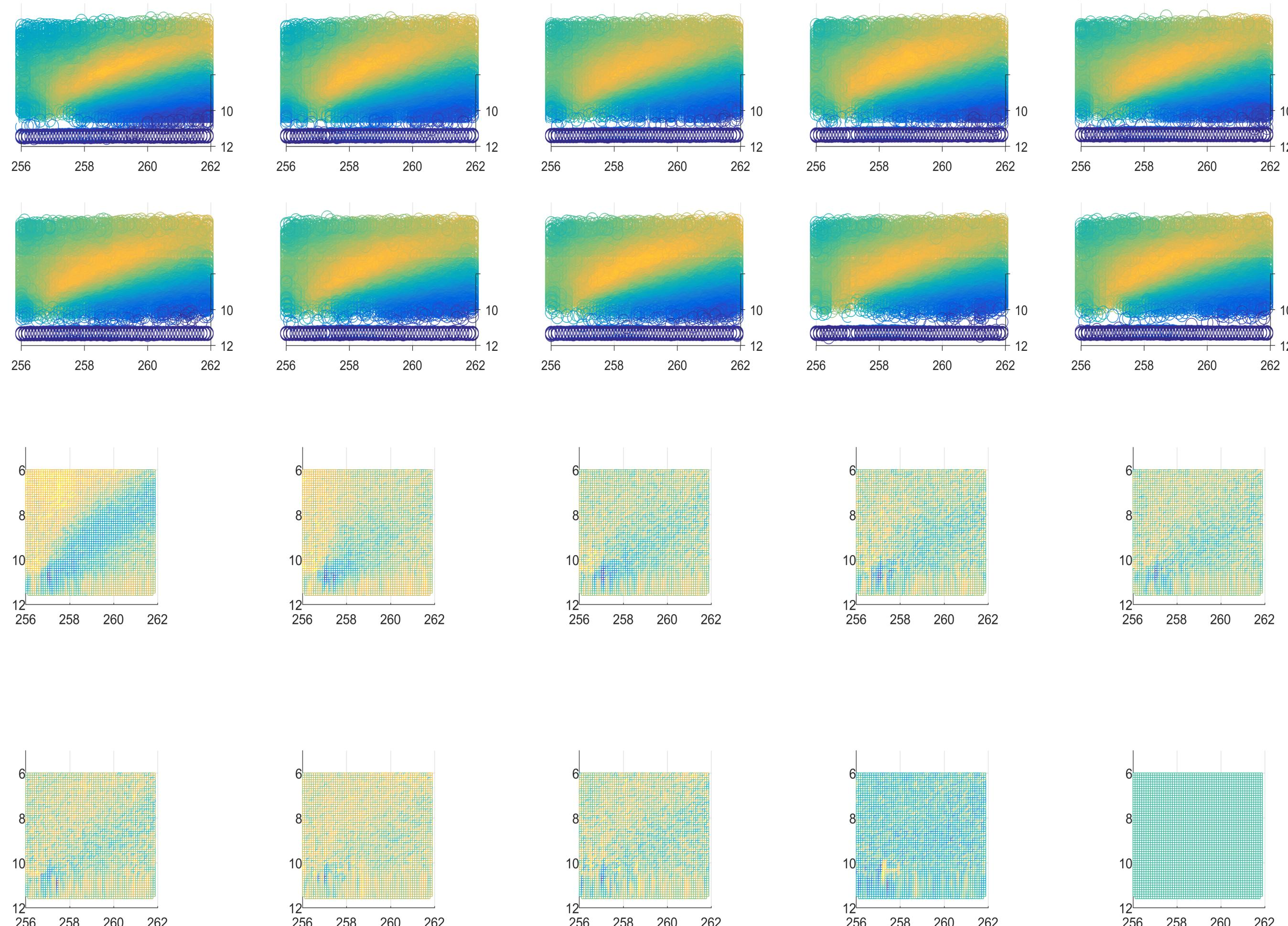
The two top rows show a set of such measurements taken over a two hour period. The bottom two rows show the difference of each plot with the last one measured. From these results we can conclude that overall, the measurement is quite stable. The first measurement shows a slightly larger Q factor, while the one-but last measurement shows a slight overall difference in amplitude level, but otherwise changes between plots are around the noise level of the measurements.
