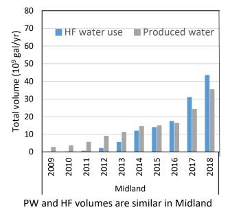
3a. Potential for Reusing Produced Water for Hydraulic Fracturing
