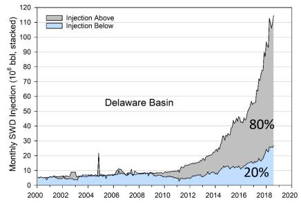
Similar trends in Midland Basin, 70% shallow, 20% deep Predominance of shallow disposal should minimize induced seismicity but could result in GW contamination from overpressuring
