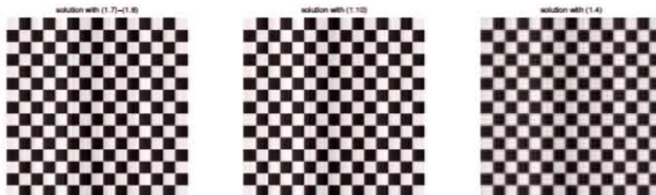
Figure: Solutions for a 2D deconvolution problem with low frequency noise. The relative reconstruction error to Tikhonov solution in standard form are  $\hat{r}e = 0.36$  and  $\tilde{r}e = 0.48$ , respectively.
