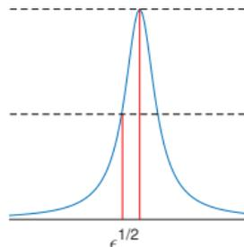
Solution  $u$  must be accurate to within  $\sqrt{\varepsilon}$  to resolve diffusion coefficient near peak!
