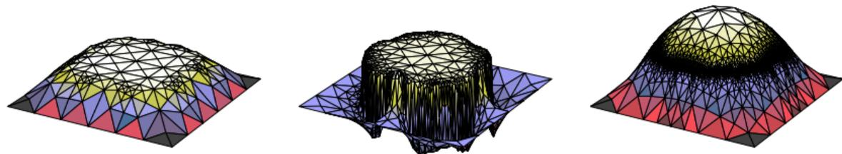
Figure: Three phases of the solution process: Level 5 with 166 dof; Level 15 with 827 dof; Level 25 with 3802 dof. Runtime to residual convergence: < 1 min.
