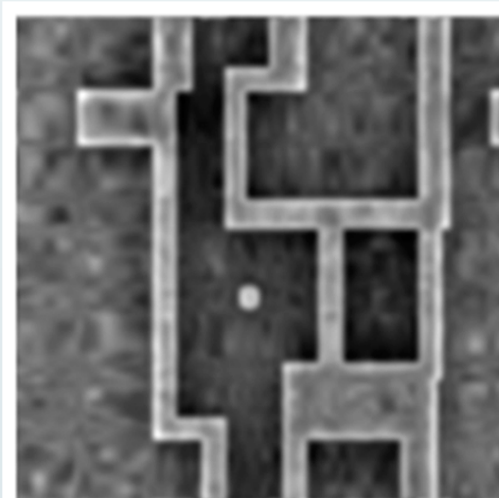
JMONSEL simulation of an intentional defect pattern
