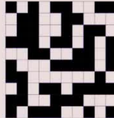
Example 2: Population on a 10x10 grid with 3 connected components and 3 holes ( \beta_0 = 3 and \beta_1 = 3 )
