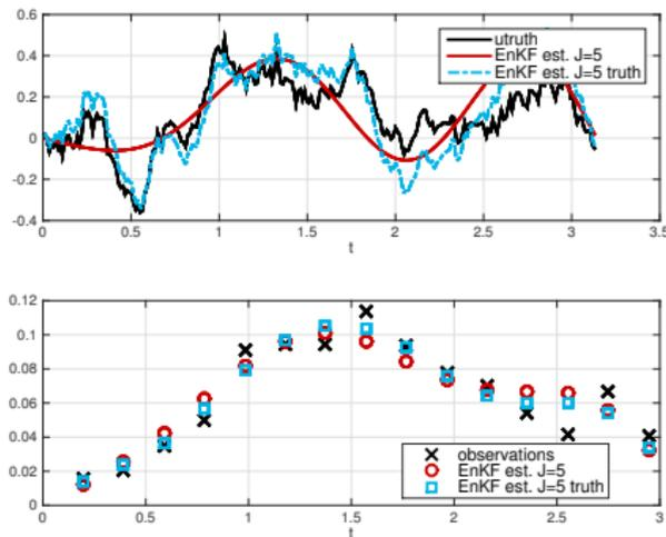
Figure: Comparison of the EnKF estimate with the truth and the observations,  $J = 5$  based on KL expansion of  $C = \beta(A - id)^{-1}$  (red),  $J = 5$  adaptively chosen (blue),  $\beta = 10$ ,  $K = 2^4 - 1$ .
