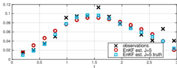
Figure: Comparison of the EnKF estimate with the truth and the observations,  $J = 5$  based on KL expansion of  $C = \beta(A - id)^{-1}$  (red),  $J = 5$  adaptively chosen (blue),  $\beta = 10$ ,  $K = 2^4 - 1$ , Bayesian stopping rule.
