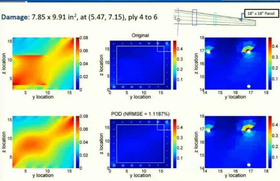
measure strain data → POD + SOM models → estimate Failure Index (FI)
