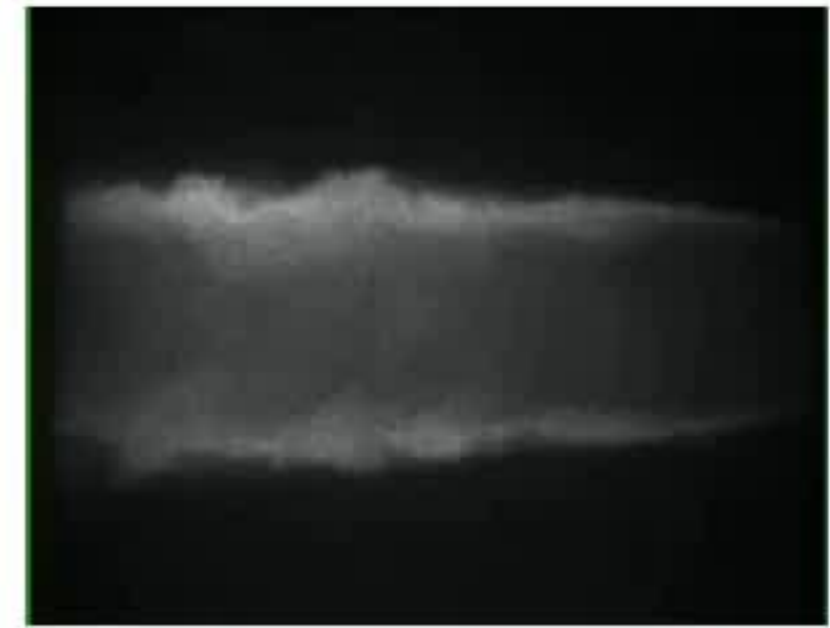
Combustion flow behind a V-shaped bluff body
