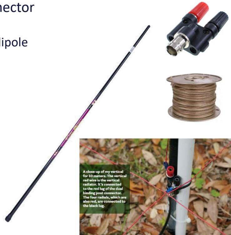
My homemade vertical for the 10-meter band. It's easy to make from 22 AWG wire. A 1/4-inch PVC tube is holding up the 13-foot collapsible fishing pole that serves as the antenna mast.
