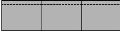
(a) Squat, shear-dominated wall, showing control joints
