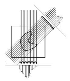
The principle in parallel-beam tomography: send parallel rays through the object at different angles, measure the damping.
