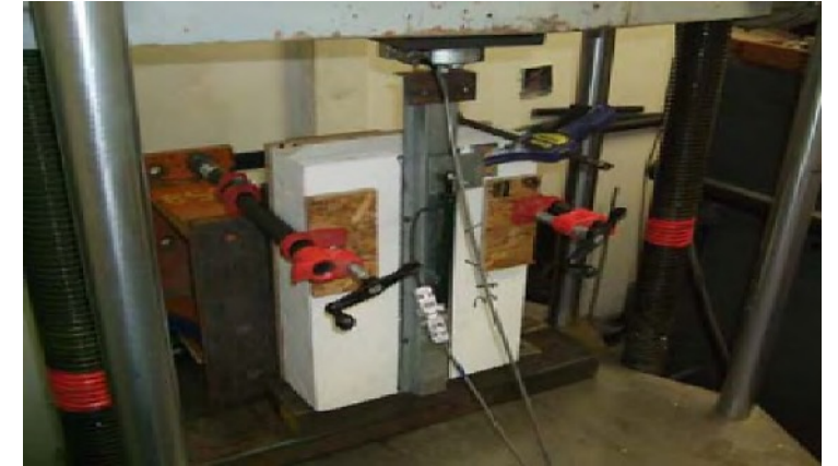
Short-term load-deflection test
