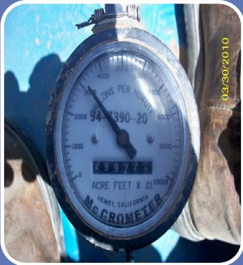
Ensure diverters have a working measuring device on-line during operation. A meter must be inspected and verified by the watermaster program before it may be used to divert water.
