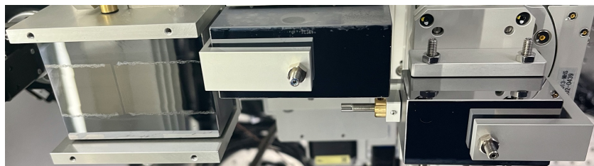
Advanced Wolter type KB mirror for 17.5 keV X-ray
